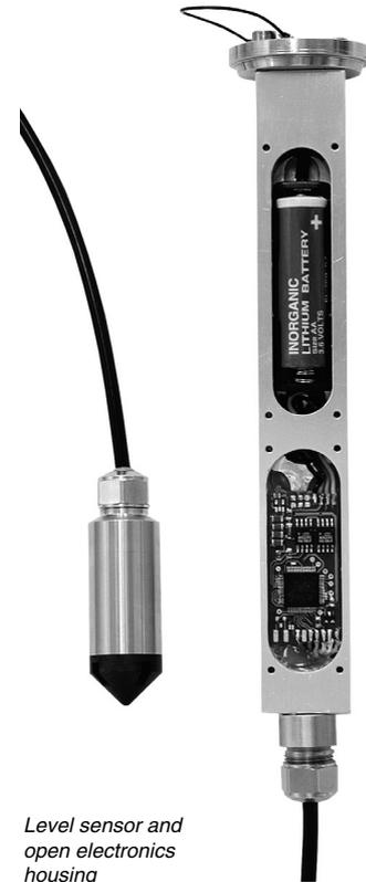
*Level sensor and open electronics housing*
